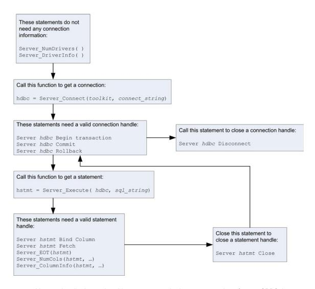
You can download an entire table, some rows and columns, or a result set from an ODBC data source using the **Into** feature of the MapBasic statement **Server Fetch**. However, any updates applied to the downloaded table are not applied back to the server database table. Updating remote databases is accomplished by the **Save File** statement.
